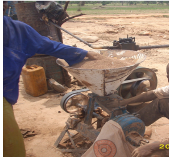
Figure 2. A flour mill was being used to process gold ore. Gold ore processing became an important source of income for the primary pastoral communities in Zamfara State.
