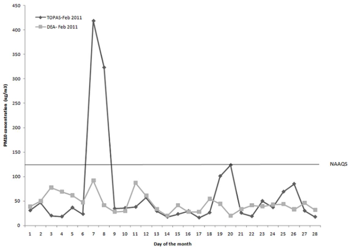
**Figure 2:** 24-hour PM10 averages monitored with the TOPAS monitor and by DEA monitoring station in summer (February 2011)
